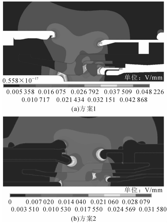
图3 大喷嘴打开时方案1与方案2灭弧室电场分布 Fig. 3 The electric field distribution in scheme 1 and scheme 2 arc extinguishing chamber at the time of large nozzle opening
